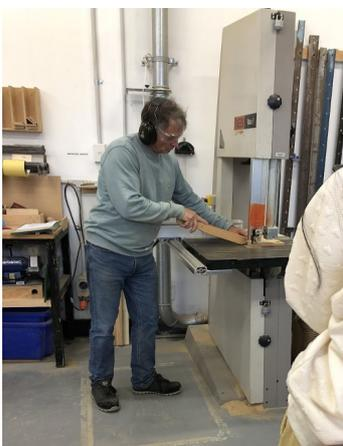
Because we all finished our boxes half an hour before the class finished, we all then got a turn being inducted into using the bandsaw. Most important things to remember for this were to use the pushing stick in order to avoid getting any fingers chopped off. The most key thing in actually cutting wood on it was to not take sharp corners, but rather carve bits off one at a time. The photo here is a demonstration of how to use the pushing stick before everyone's attempts.
