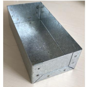
The first steps were measuring box dimensions and using the guillotine and corner cutting machine in order to get the right shape while the metal is flat. We used adjustable square rulers and tools to score the lines. The guillotine can only cut lines, not corners so we used a different machine in order to cut the pieces out to be able to bend the sheet metal.
